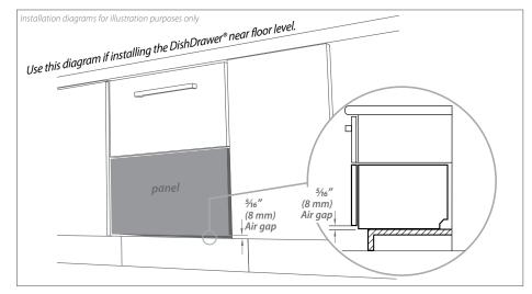
The following calculations assume the top of the panel is aligned with the top of the adjacent cabinetry:
